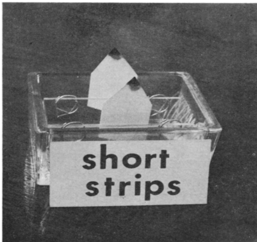
Fig. 2. Short-strip separations of organic from inorganic fluoride.
